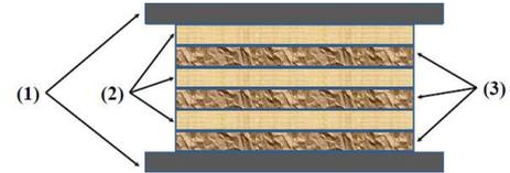
**Fig. 1.** Alternating layers of material: (1) metallic contacts, (2) high dielectric permittivity layers, and (3) high breakdown voltage materials.
